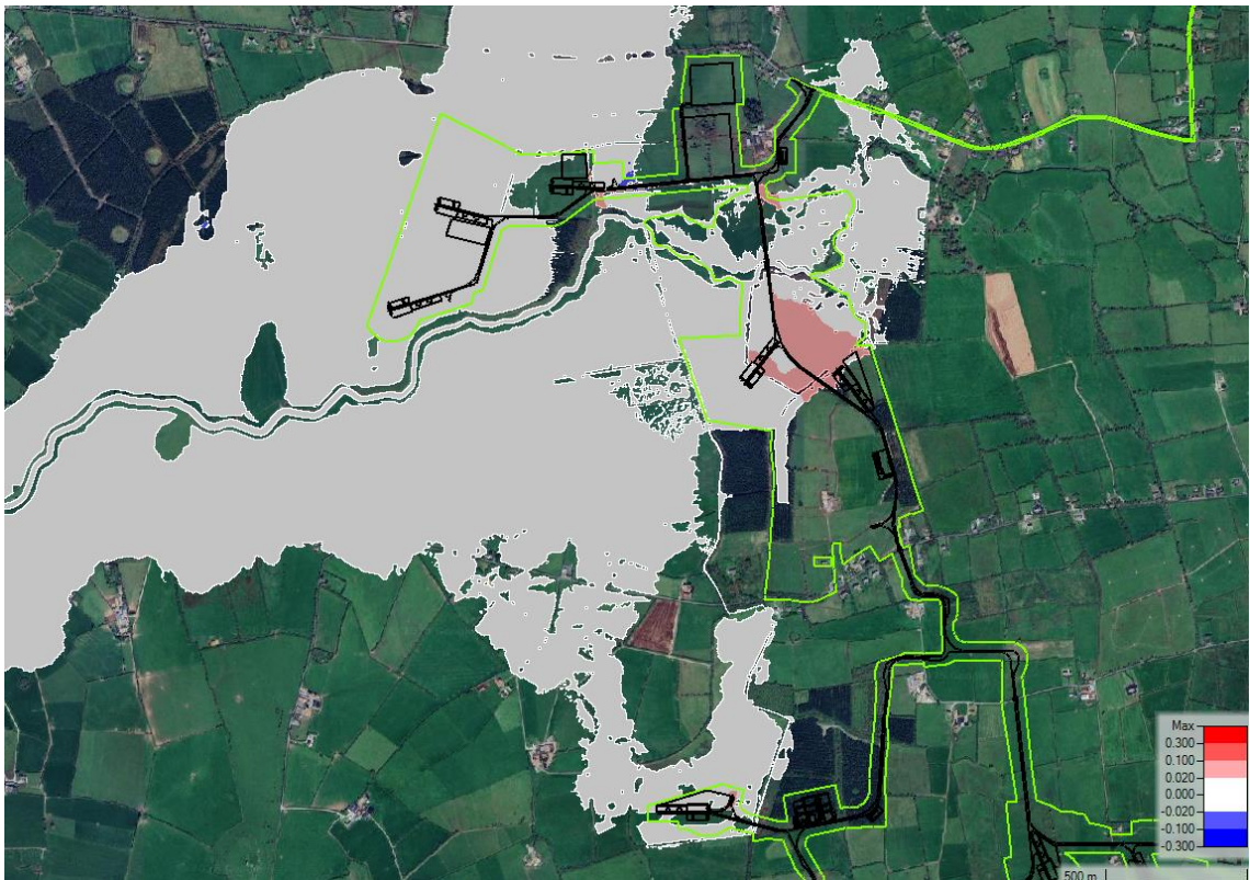
Figure 4.20: Flood Level Comparison - Baseline v Proposed - 1% AEP MRFS
