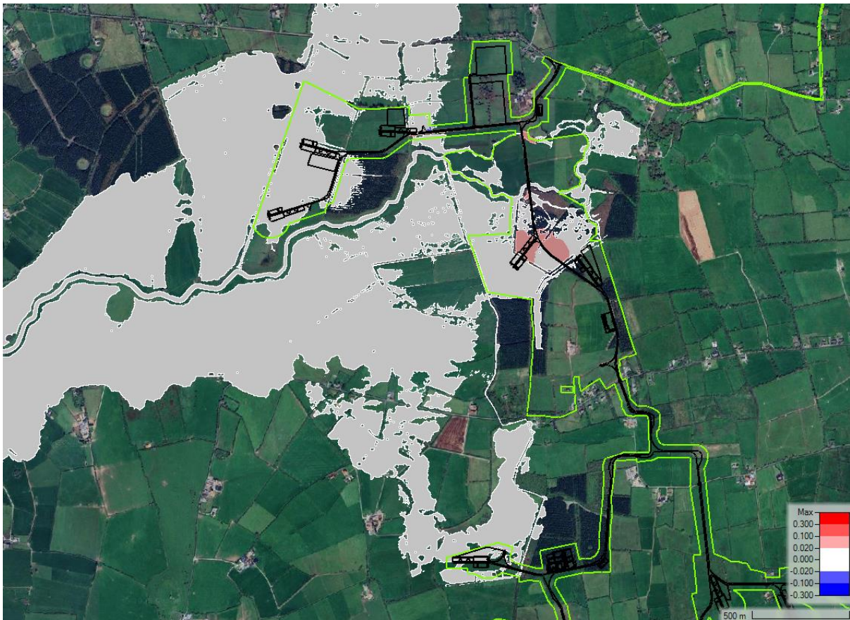
Figure 4.18: Flood Level Comparison - Baseline v Proposed - 5% AEP
