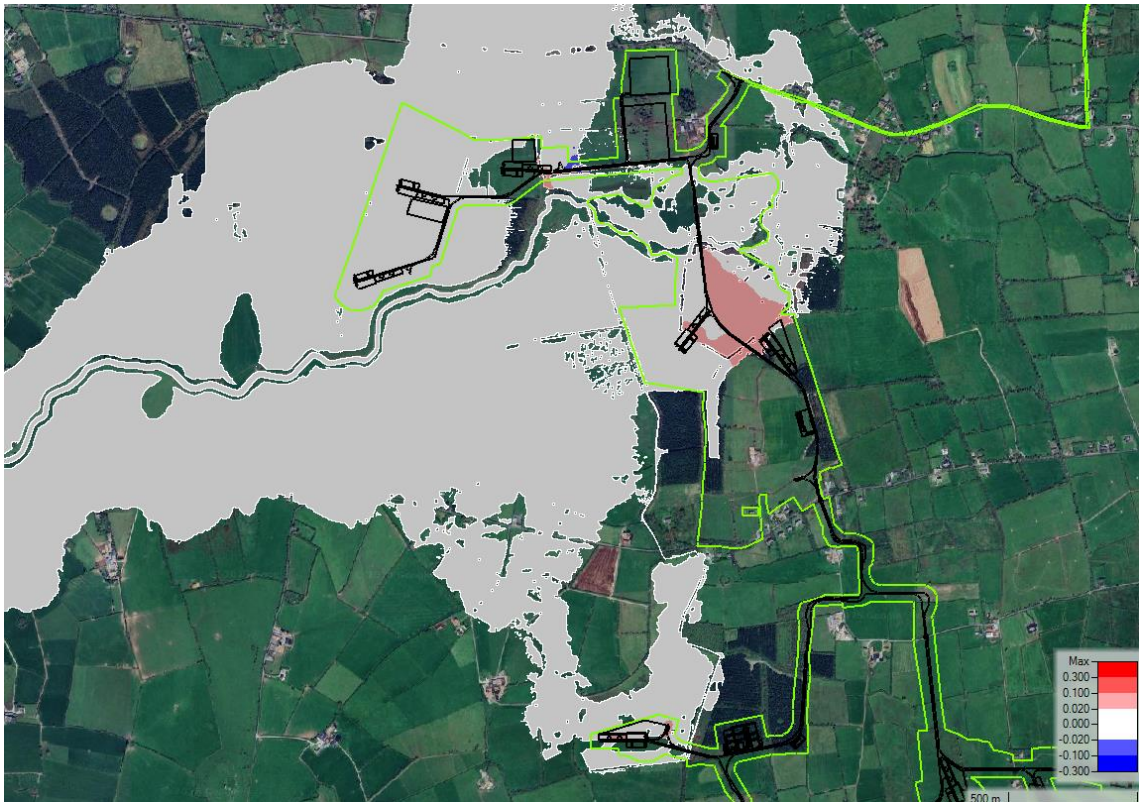
Figure 4.20: Flood Level Comparison - Baseline v Proposed - 1% AEP MRFS
